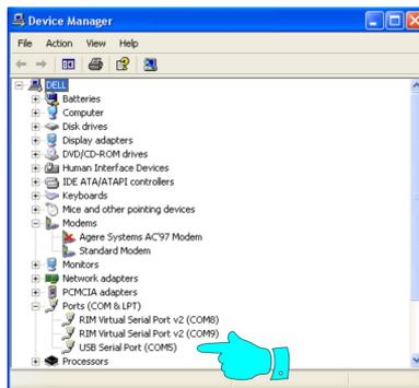
Use this port to manually assign the COM port in the Acuity Pro control panel.
